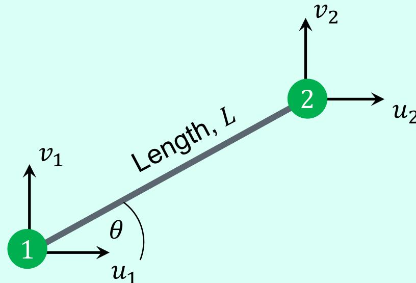
Only displacements parallel to bar axis cause extension/compression
